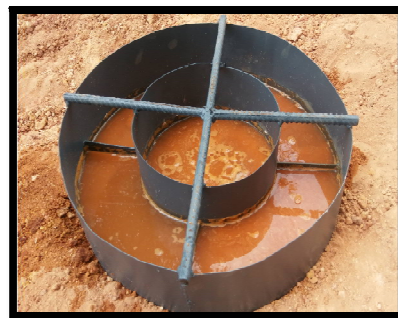
Figure 1: Double Ring Infiltrometer
